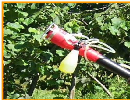
Figure 1. Air-assisted rotary disc nozzle
