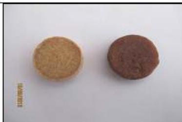
Figure 3: Effect of water activity on color stability of tablets (left: original color).
